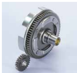
202.1216 Vespa 50 75/90 Z=24/72 Primary ratio-Primario
