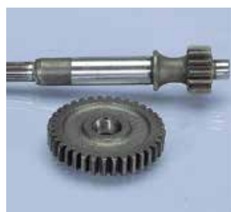
202.1334 Cagiva City Z=17/41 Primary ratio-Primario
