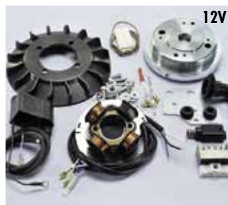
171.0545 Vespa 125 ET3 cone/cono Ø19, flywheel/volano 1,2Kg
