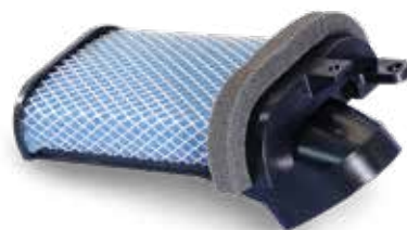
203.0154 TMAX 500-530 variator cooling filter Raffreddamento variatore TMAX 500-530
