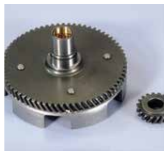
202.1218 Vespa 50/75 Z=18/67 Primary ratio-Primario
