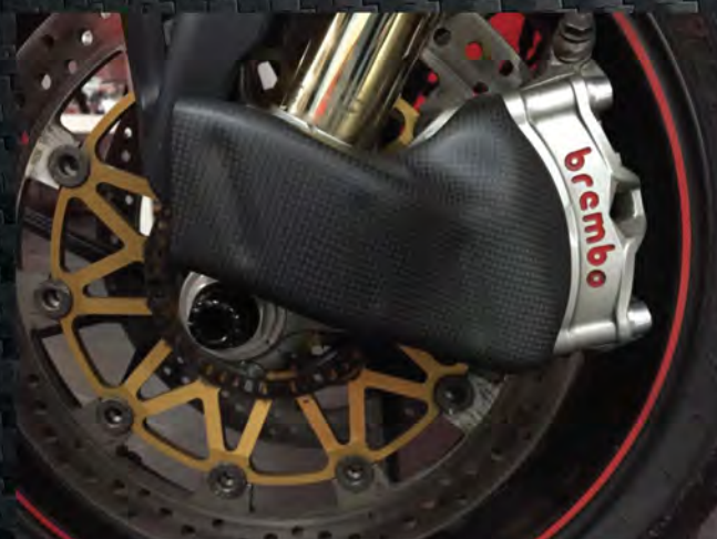
Brake caliper air duct.
