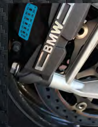
Brake caliper prepared with temperature stickers.
